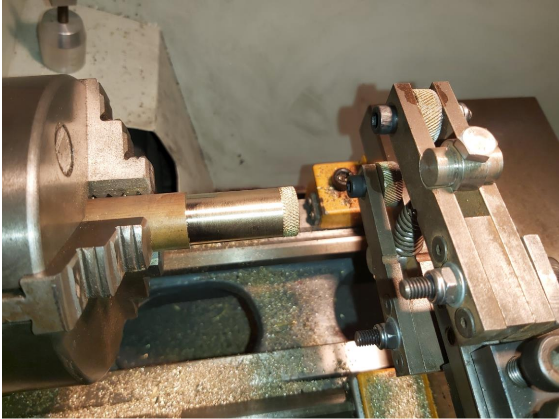
A 6mm gripping ridge was knurled on this lathe.
